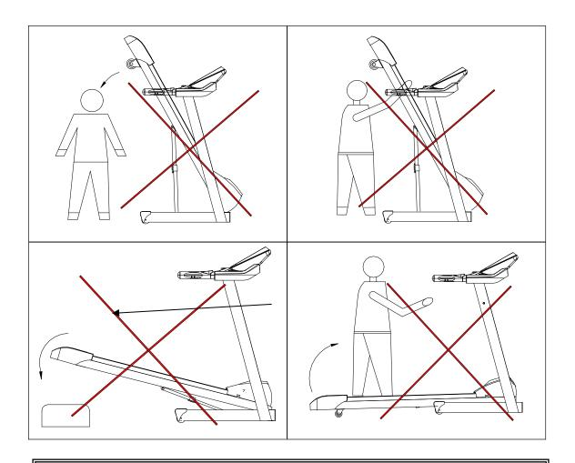
WARNING 2: Make sure the treadmill has been disconnected with the electricity. You can switch off the treadmill by pressing the main power switch as below.
