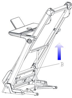
STEP 7: With one hand at position A, kick the air pressure rod with your foot, and press down
