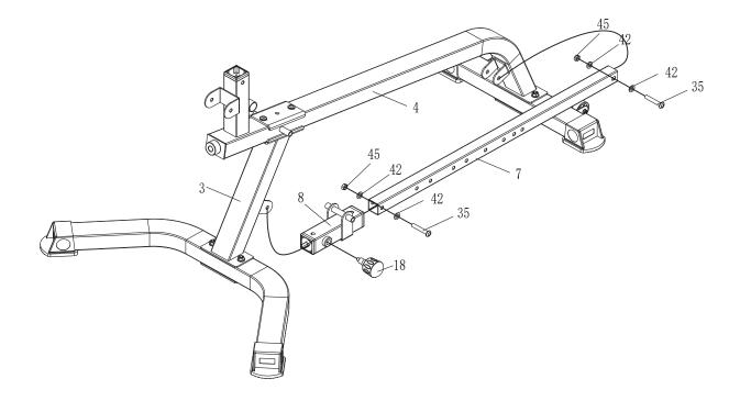
1. Align the seat/cushion main frame (4) and the seat cushion frame (5) with the holes in accordance with the picture, and use M10\*195 hexagon socket pan-headed bolts (38),  $\Phi$ 10 flat pads (42) and M10 jam nut (45) to fix and fasten.
